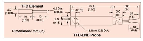
Voltage Necessary for Destruction: 100 Vdc Hysteresis Error (Observed Only after Rapid Temperature Cycling): Max 0.25 Self-Heating Error at 20°C (70°F):
